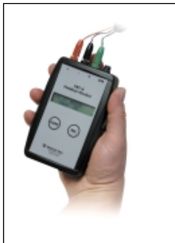
Figure 2: Typical hand-held fieldbus monitor
